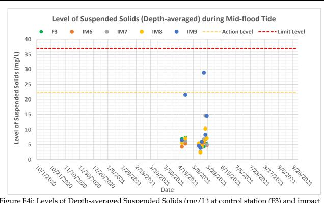
Figure F4i: Levels of Depth-averaged Suspended Solids (mg/L) at control station (F3) and impact stations (IM6-IM9) under Group 3 during mid-flood tides between October 2020 and September 2021
